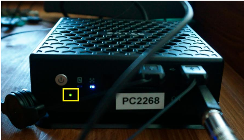
Figure 3 – mini PC from inside the interactive table in power on mode.
